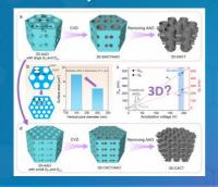
A simple technique is achieved to finely adjust the vertical-pore diameter and interspacing in three-dimensional nanoporous anodic aluminum oxide (3D-AAO) template, and 3D compactly arranged carbon tube (3D-CACT) nanoarrays was created as electrodes for symmetrical EDLCs using nanoporous 3D-AAO template-assisted chemical vapor deposition of carbon.
